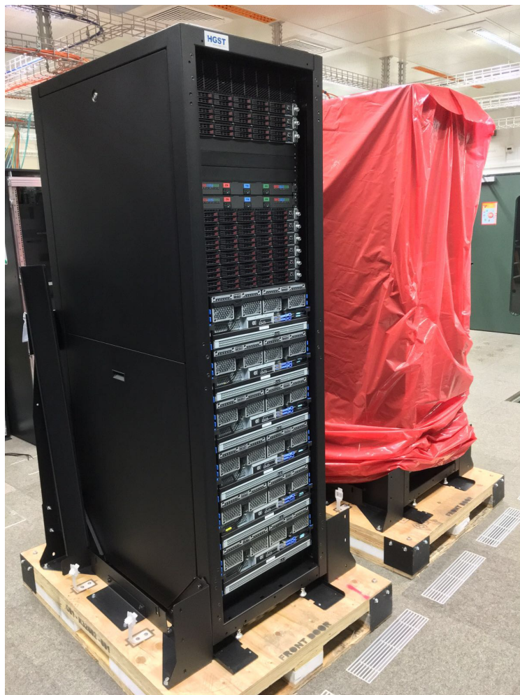
Five racks of hard-drives from Amplidata storing the MJF Archive in the datacenter of EPFL in 2015 (above), and two of the new 4.7PB Active Archive units from HGST, just arrived at EPFL in February 2016 (below).
